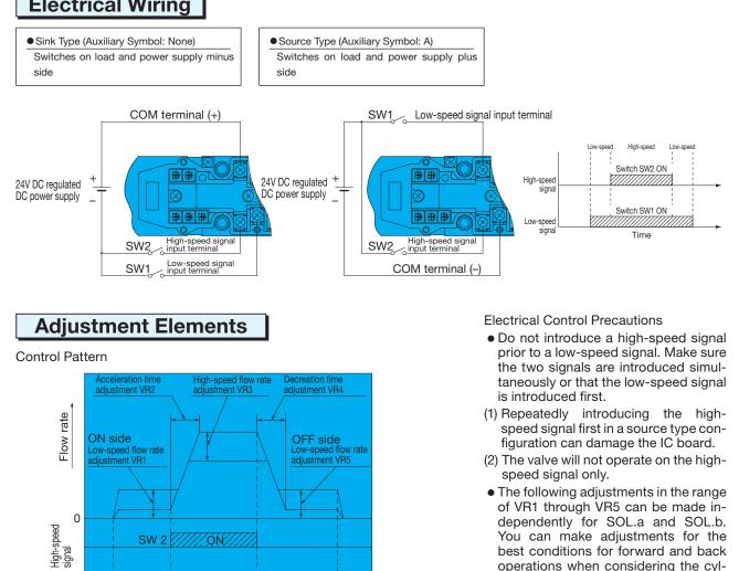
dependently for SOL.a and SOL.b. You can make adjustments for the best conditions for forward and back operations when considering the cylinder operations.
