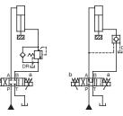
When large brake pressure is required (Use an external drain type counter valve.) When there is the possibility of pilot check valve knocking (Use an external drain type pilot check valve.)
